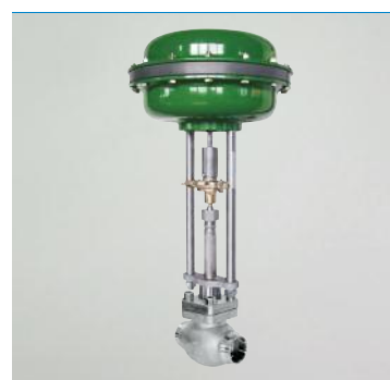
ESD Pneumatic Actuated Globe Valve Materials: Bronze / Stainless Sizes: 1/2"-6" / 15-150mm Pressures: 720psi / 50 bar Temperatures: -321°F to +248°F / -196°C to +120°C Connections: Threaded, SW, BW, Stubbed, Flanged
