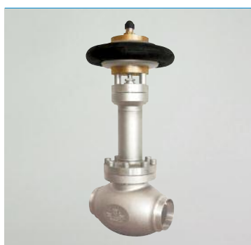
ESD Pneumatic Actuated Globe Valve Materials: Stainless Sizes: 1.1/2"-3" / 40-80mm Pressures: 145psi / 10 bar Temperatures: -321°F to +248°F / -196°C to +120°C Connections: SW, BW
