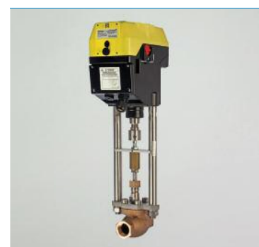
ESD Electrically Actuated Globe Valve Materials: Bronze / Stainless Sizes: 1/2"-6" / 15-150mm Pressures: 720psi / 50 bar Temperatures: -321°F to +248°F / -196°C to +120°C Connections: Threaded, SW, BW, Stubbed, Flanged
