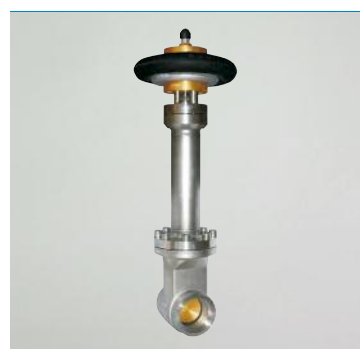
ESD Pneumatic Actuated Gate Valve Materials: Stainless Sizes: 1"-4" / 25-100mm Pressures: 720psi / 50 bar Temperatures: -321°F to +248°F / -196°C to +120°C Connections: SW, BW
